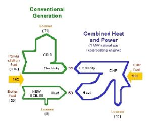
CHP is not a single technology but a suite of power generation technologies (engines, combustion turbines, microturbines, steam turbines, sterling engines and fuel cells) that can use a variety of fuels to generate electricity or mechanical power at the point of use, and allow utilization of the thermal energy from the power generation equipment, for providing heating and/or cooling needs of the facility by using a variety of heating and cooling equipment.
